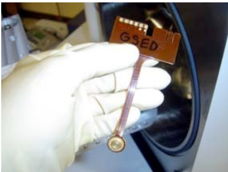
Figure B1. Gaseous Secondary Electron Detector (GSED).
