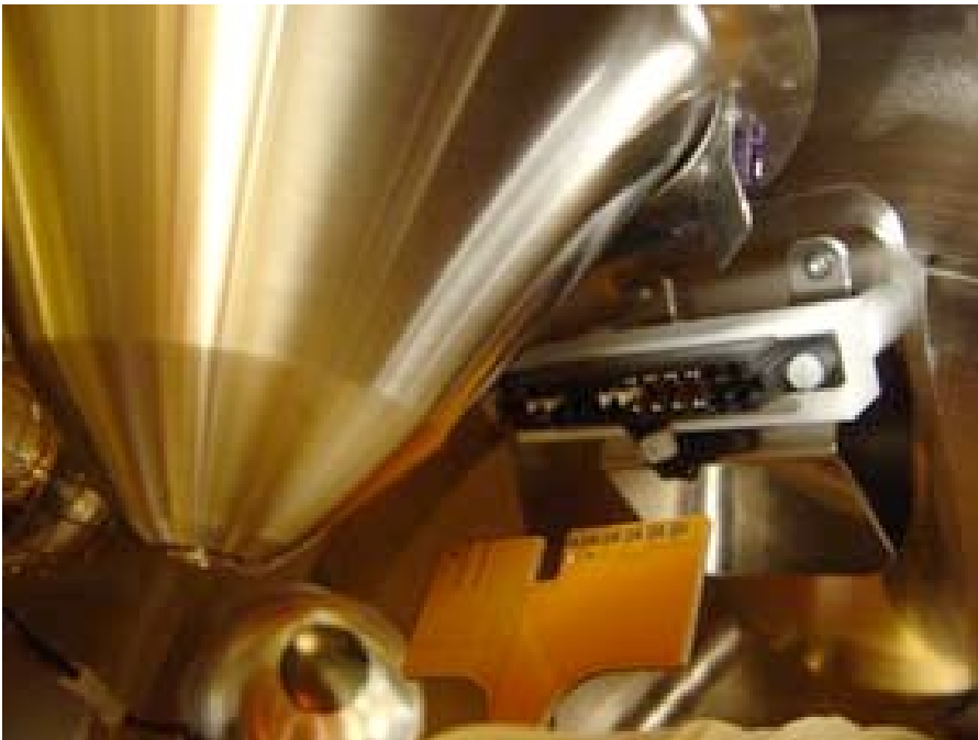
Figure A2. Installing the LFD or GSED into the connector in the rear of the chamber can be awkward; be sure to match up the slots in the card with the connector properly.
