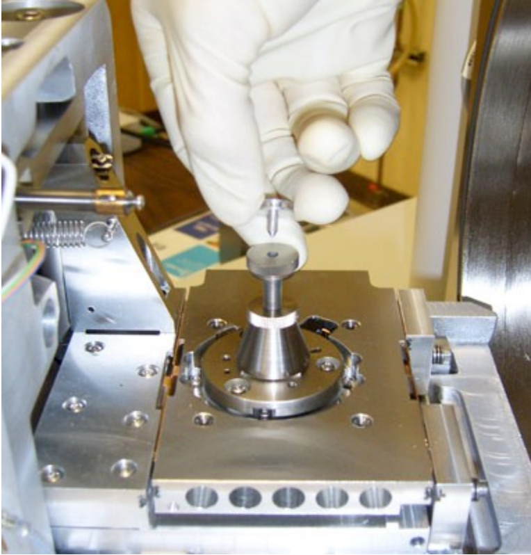
Figure 5. Inserting the specimen stub into the stage.
