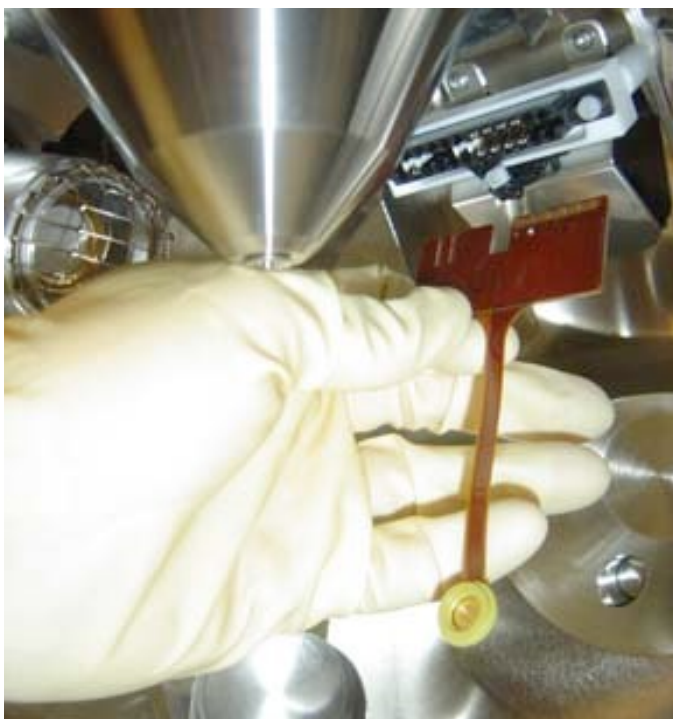
Figure B2. Inserting the GSED card into the connector slot.
