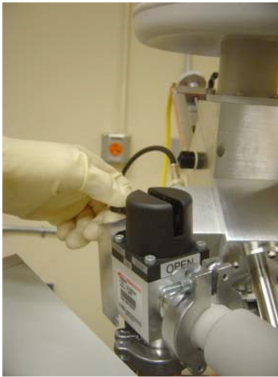
Figure A4. Open the environmental backing valve (EBV) only when prompted by the computer system.
